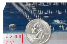
9.5 mm Bashplate Protects LED and Internal Components
