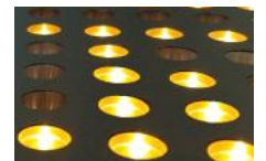
Individual cones for each LED
